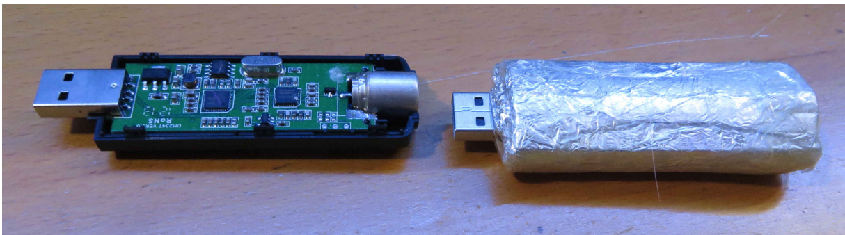
Picture 11: The dongle opened (left) and shielded (right)
