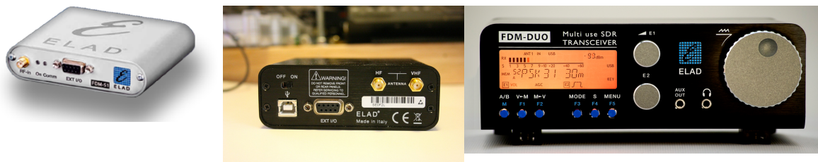
Picture 12: Three ELAD devices: left to right, samplers S1 and S2, transceiver FDM DUO
